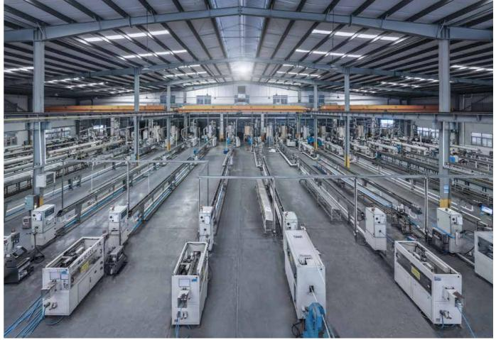
RIIFO PEX pipes automated production lines
